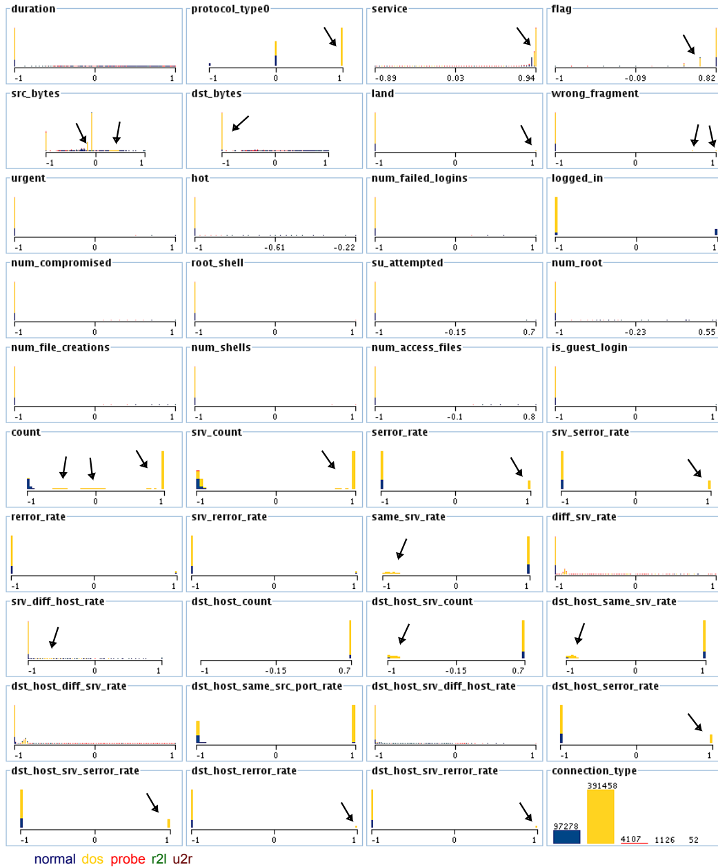
Figure A.2: Distributions histograms of all features in the preprocessed KDD Cup '99 '10% training data. The x-axis shows the value of the feature and the y-axis shows how often the value exists in the training data. The highlighted features strongly correlate with the 'dos' attack class.
