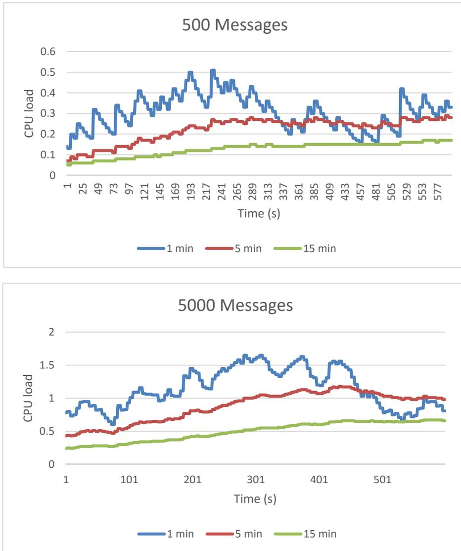
**Figure 59: CPU load for the traffic application in the three different scenarios including 50, 500 and 5000 messages per 30 second interval.**
