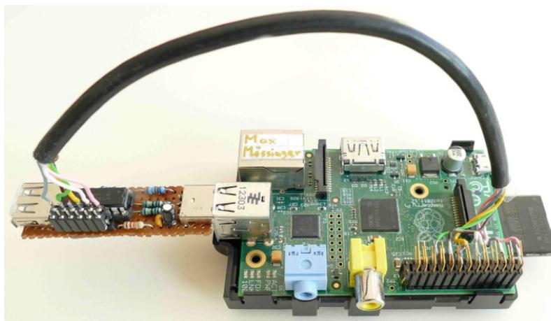
**Figure 7: USB stick to measure energy consumption of the RE-Mote connected to a Raspberry Pi [M16].**
